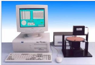
Fig.3 Resist thickness measurement system.
