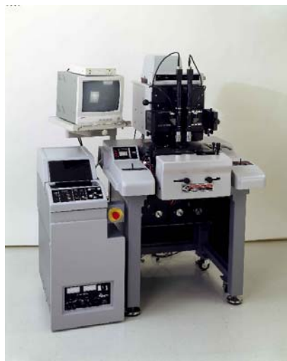
Fig.9 Mask aligner of the proximity printing type.
