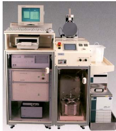
Resist development rate measurement system: RDA
